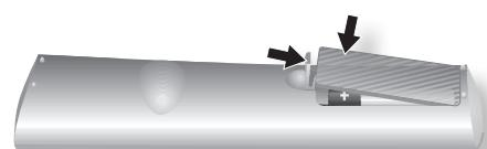
3. Replace the battery compartment cover, locking the tab with a click.
