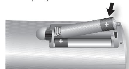
2. Insert the two 'AAA' batteries supplied in the proper direction, following the '+' and '-' marks in the battery compartment.
