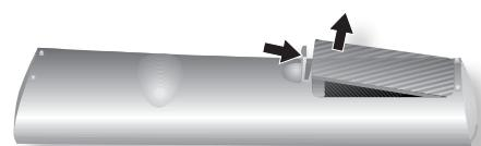
1. Squeeze the tab and lift off the remote control's battery compartment cover.
